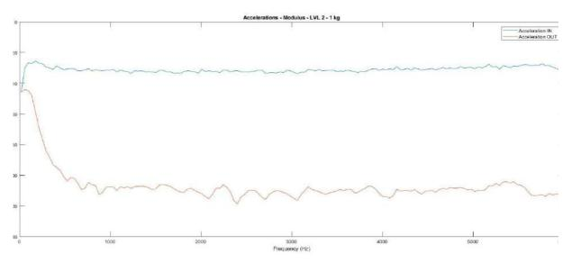
Figure 4. Incoming and outcoming accelerations on Level 2 damper loaded with 1 kg.
