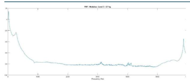
Figure 9. FRF on Level 3 damper loaded with 3.7 kg.
