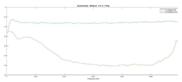
Figure 6. Incoming and outcoming accelerations on Level 4 damper loaded with 7.4 kg.
