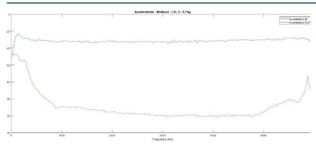
Figure 5. Incoming and outcoming accelerations on Level 3 damper loaded with 3.7 kg.
