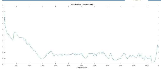
Figure 11. FRF on Level 5 damper loaded with 13 kg.
