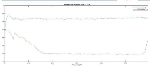
Figure 7. Incoming and outcoming accelerations on Level 5 damper loaded with 13 kg.
